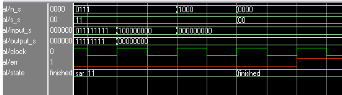
FIGURE 3.1.2: ERR (in red) is asserted and state is set to ‘finished’ when the list of all possible inputs is exhausted.
