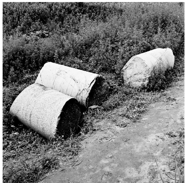
Fig. 5. Borehole core of the granite rock in the dam site (core diameter is 800 mm).
