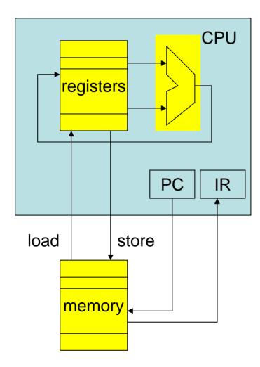
• **RISC** architectures are load/store. The regularity of this architecture enables fast organizations using pipelining (Appendix A).
