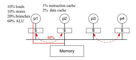
We assume the simple write-through invalidate snooping protocol where every store operation places the address of the block on the bus and cache controllers snoop on the bus and invalidate their block if it was originally in their cache.
