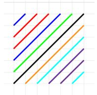
The advantage of such a method is that besides synchronization, there is no need for communication between the processors. By looking at the figure, if we assume that every grid intersection is a matrix value, we can see that all processors (represented by different colors) share an equivalent work load (in this case, every processor will do 6 swaps, since the central elements on the diagonals don't need to move).
