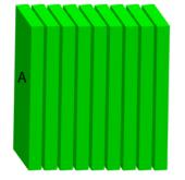
In this case, every sub domain has 2 sides for communication area of size  $n^2$ , so the total communication area per processor is  $2n^2$ . This makes the CCR  $[2n^2] / [n^3/p] = 2p/n$
