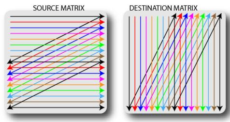
In the initial matrix, a processor would commit to transposing a particular row into a particular column in the target matrix. Whenever a process is done, it could go ahead and commit to the next available row/column pair until the entire matrix has been processed.
