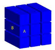
In this case, the area of every sub domain is composed of 2 sides (A) of  $n^2/p$  and 4 sides (B) of  $n^2/vp$ . It is important to observe that no matter how large n or p, the sides 'A' will never have to make any kind of communication between processor, the communicating areas is only composed of 4 \*  $n^2/vp$ This scheme would yield a CCR of [4 \*  $n^2/vp$ ] /  $[n^3/p] = 4vp/n$
