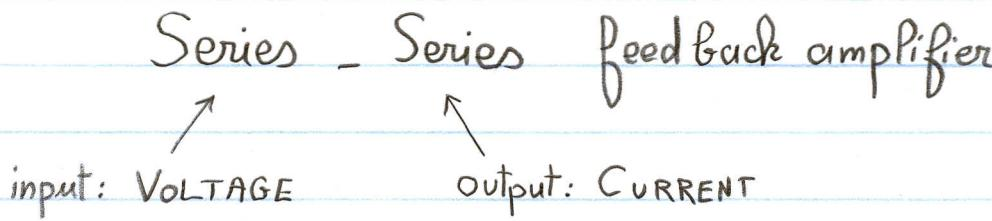
input: VOLTAGE      output: CURRENT
