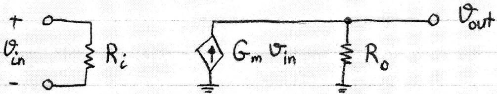
$$\cdot A_v \triangleq \left. \frac{v_{out}}{v_{in}} \right|_{R_L=\infty} = G_m R_o = (g_{m1,2}) \left( \frac{1}{3} \beta R_o \right)$$
