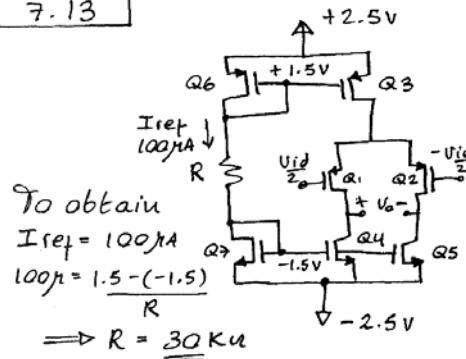
$$V_{GS,7,4,5} = -1.5 + 2.5 = \underline{\underline{1V}}$$
