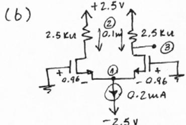
$$\begin{aligned} (1) \quad V_{S1} &= V_{S2} = V_{CM} - V_{GS} \\ &= 0 - 0.96 = -0.96V \end{aligned}$$
