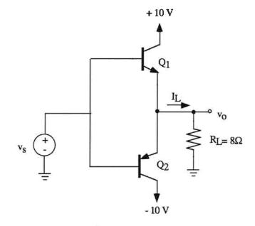
(b) A modified class B BJT power amplifier of the type shown in the figure to the right is driven by a sinewave input of 10 V peak centered around 0 V.
