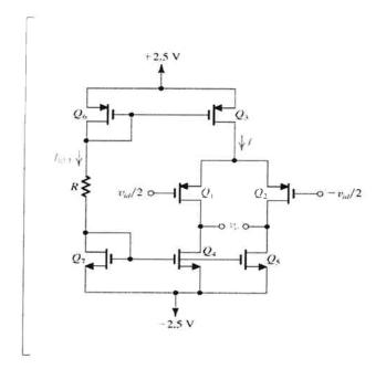
The circuit on the left shows a circuit for a differential amplifier with an active load. Here  $Q_1$  and  $Q_2$  form the differential pair while the current source transistors  $Q_4$  and  $Q_5$  form the active loads for  $Q_1$  and  $Q_2$ , respectively.
