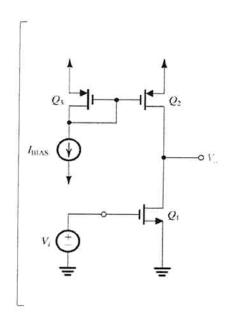
It is required to analyze the high-frequency response of the CMOS amplifier shown to the left. The DC bias current is set to  $50 \, \mu A$ .
