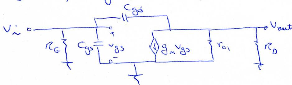
b) mid-band gain :  $\left\{ \begin{array}{l} C_S \text{ and } C_C \rightarrow S.C. \\ C_{GS} \text{ and } C_{GD} \rightarrow O.C. \end{array} \right.$
