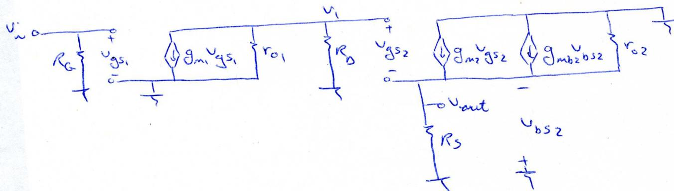
$$d) g_m = \frac{2I_{D_1}}{V_{GS1} - V_{tn}} = \frac{2 \times 0.5 \text{ mA}}{0.5^{\circ}} = 2 \text{ mA/V}$$
