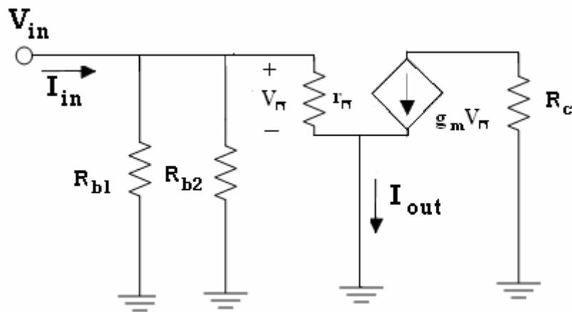
$$i_{in} = \frac{v_{in}}{R_{b1} \parallel R_{b2}} + \frac{v_{in}}{r_\pi}$$
