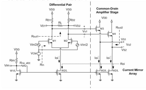
Neglect the Body effect. You must include CLM output resistances for the current mirror but neglect CLM elsewhere. Assume  $V_{DD}$ =1.8V and  $R_{D1}$  =  $R_{D2}$ .
