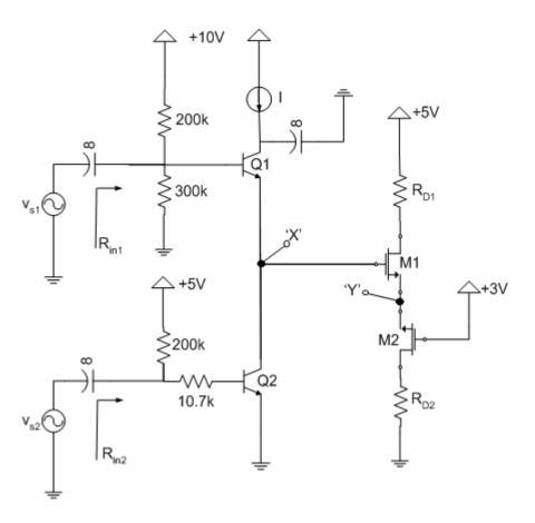
a) [2 pts] Assuming the BJT's have  $\beta$ =99,  $|V_{BE}|$  = 0.7V and I = 2mA, determine  $V_X$ , the DC voltage at node X.
