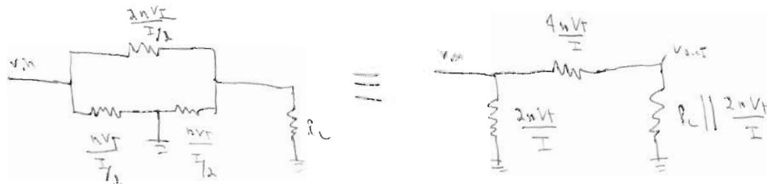
$$\frac{V_{out}}{V_{in}} = 0.289 \text{ V/V by analysis}$$
