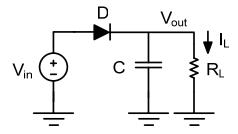
c) Plot the output voltage and find the approximate value of the ripple voltage.
