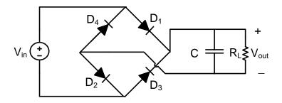
d) Plot the output voltage and find the approximate value of the ripple voltage.
