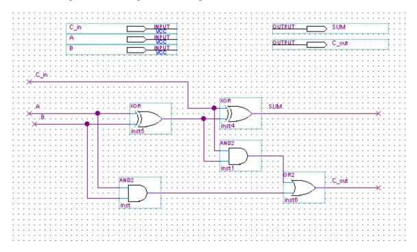
This full adder's main function is to add 3 numbers: A and B (both user specified) and  $C_{in}$ ; the carry in from the adjacent less significant bit. The sum is outputted in the SUM line, and the carry out in  $C_{out}$ .
