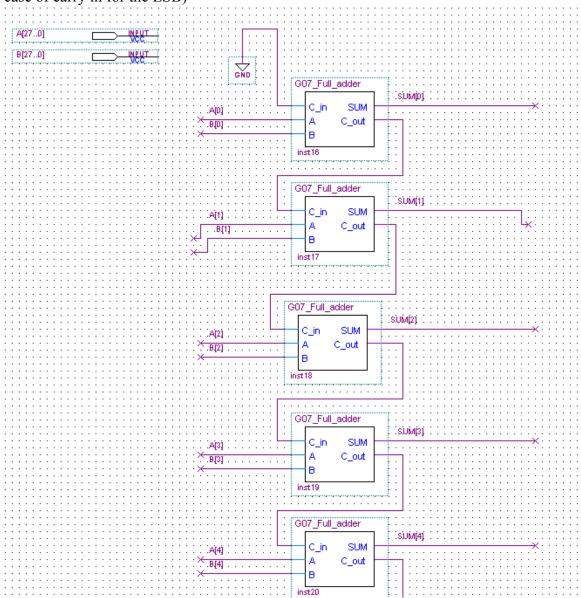
In order to build a 28 bit adder, we linked 28 of these building blocks. For the adder handling the least significant bit, the C\_in got connected to ground (since there can't be a case of carry in for the LSB)
