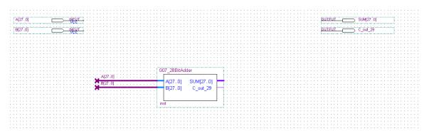
The circuit's inputs are A and B; both 28 bit bus lines to input the numbers to be added. The outputs are SUM, a 28 bit bus line to output the addition result and C\_out, a  $29^{th}$  bit to express the result of a 28 bit overflow. Note that connecting SUM to pins 0-27 and C\_out to pin 28 of a 29 bit register will generate a complete addition answer.
