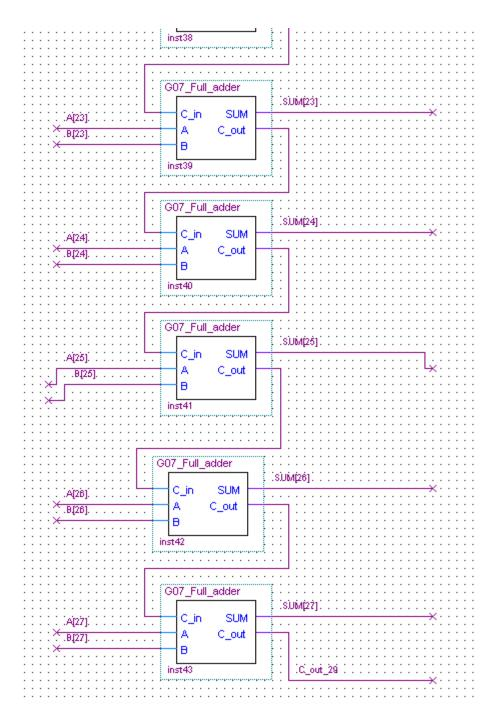
This circuit's main function is to perform the addition between two 28 bit numbers, A and B.
