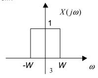
The sampling theorem is satisfied for  $\omega_s>2W$  for the first sampler. The second sampler satisfies the sampling theorem if
