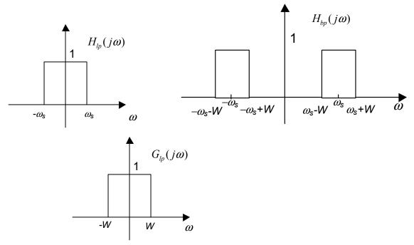
(a) [7 marks] Find and sketch  $X(j\omega)$ , the Fourier transform of the input signal x(t). For what range of sampling frequencies  $\omega_s = \frac{2\pi}{T}$  is the sampling theorem satisfied for the first sampler? What is the smallest positive integer M that will ensure that the second sampler satisfies the sampling theorem?
