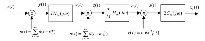
Where the input signal is the convolution  $x(t) = \frac{W^2}{\pi^2} \operatorname{sinc}\left(\frac{W}{\pi}t\right) * \operatorname{sinc}\left(\frac{W}{\pi}t\right)$  and the spectra of the ideal bandpass filter and the ideal lowpass filters are shown below.
