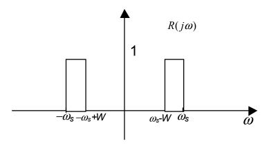
The modulation with a cosine signal makes two copies of  $R(j\omega)$ , one around  $\omega_s$  and on around  $-\omega_s$ , which reconstructs the spectrum around  $\omega=0$ :
