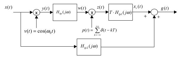
The input signal is  $x(t) = \frac{W}{\pi} \mathrm{sinc} \bigg( \frac{W}{\pi} (t - \frac{\pi}{W}) \bigg)$ , and  $\omega_0 = 2W$ .
