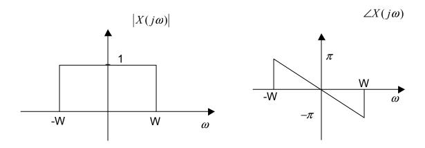
The cutoff frequencies such that  $\omega_{bp2}-\omega_{bp1}$  is minimized, and the total average power of w(t) is maximized are:  $\omega_{bp1}=W,\ \omega_{bp2}=3W$ .
