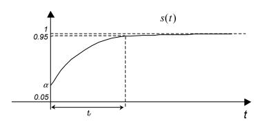
The 95% rise time is given by the difference between the times when the response reaches the value 0.95 and the value 0.05. Since  $\alpha > 0.05$ , the output is already larger than 0.05 at  $t = 0^+$ .
