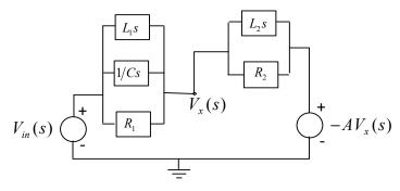
There are two supernodes for which the nodal voltages are given by the source voltages. The remaining nodal equation is
