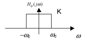
The cutoff should be between the fundamental and the second harmonic, say  $\omega_c = \frac{3\pi}{T}$ . The gain
