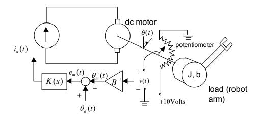
Before closing the feedback loop, we first look at the open-loop dynamics of this system in (a) and (b). The torque  $\tau(t)$  in Newton-metres applied to the load by the motor is proportional to the armature current in Amps:
