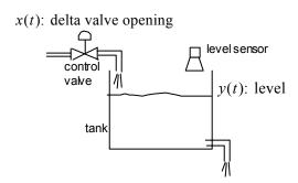
The open-loop tank dynamics are modeled by the following nonminimum phase transfer function
