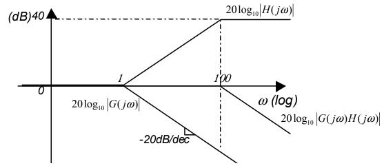
The circuit must be a first-order lead with a transfer function of the form
