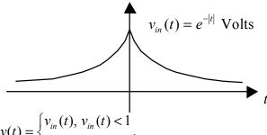
and the output voltage is  $v(t) = \begin{cases} v_{in}(t), v_{in}(t) < 1 \\ 1, v_{in}(t) \ge 1 \end{cases}$
