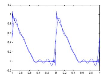
The fifty-harmonic approximation is obviously a better representation of the sawtooth waveform, but significant ripple are seen in the plots of both truncated Fourier series, especially around the discontinuities.
