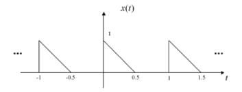
Figure 4.12: Periodic sawtooth signal in Exercise 4.8(a).
