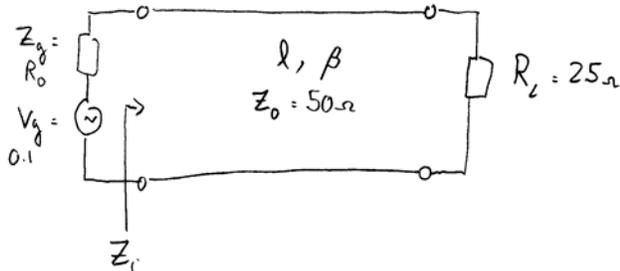
$$(a) \quad Z_i = R_0 \left[ \frac{R_L + R_0 j \tan \beta l}{R_0 + R_L j \tan \beta l} \right]$$
