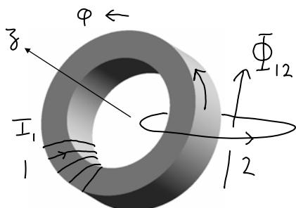
$\underline{B}_1$  is zero outside the toroid, so the flux  $\Phi_{12}$  passing through coil 2 is just the flux flowing around inside the toroid.
