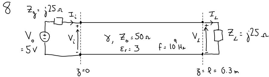
$$\text{Lossless} \Rightarrow \gamma = j\beta \quad \beta = \omega \sqrt{LC} = \omega \sqrt{\frac{\epsilon_r}{C}} = \frac{2\pi f \sqrt{\epsilon_r}}{l} = \frac{20\pi}{3} = 36.28 \text{ rad/m}$$
