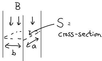
$$\Rightarrow \text{Flux } \Phi = \int_S B \cdot dS = BS = \left( \mu \frac{N_1 I}{4D} \right) ab$$
