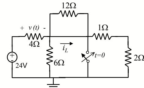
→ 12Ω resistor is shorted out by the inductor.
