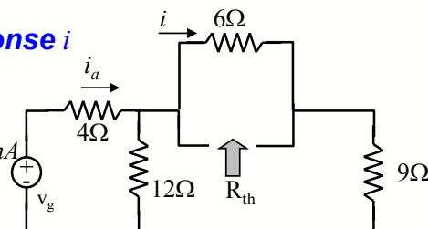
$$R_{th} = (4\Omega \parallel 12\Omega + 9\Omega) \parallel 6\Omega = 4\Omega$$
