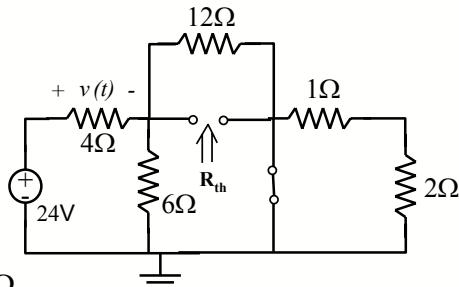
$$R_{th} = 4\Omega \parallel 6\Omega \parallel 12\Omega = 2\Omega$$
