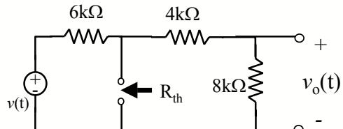
$$R_{th} = 6k\Omega \parallel (4k\Omega + 8k\Omega) = 4k\Omega$$
