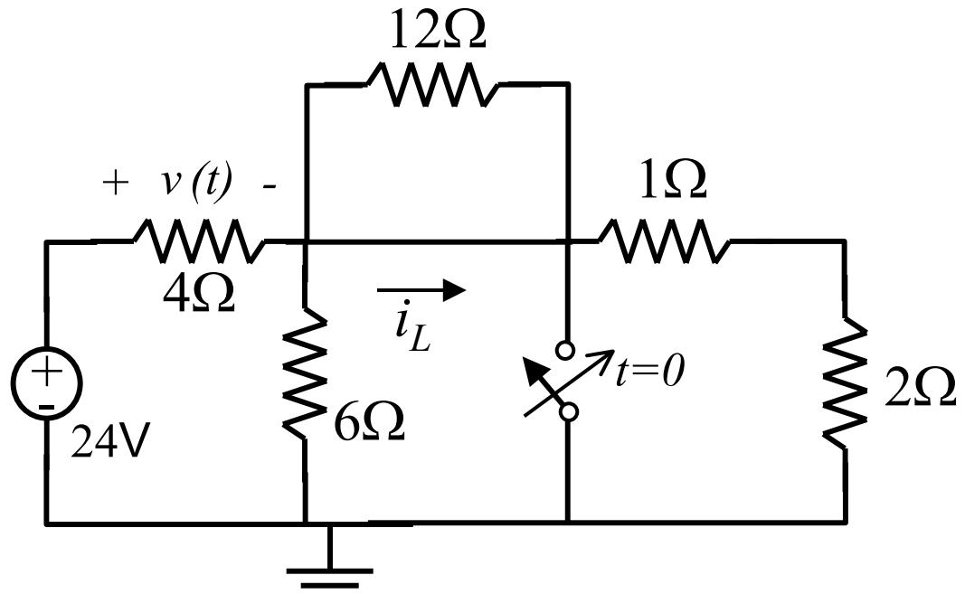
$$v(t) = \frac{4\Omega}{4\Omega + 6\Omega \parallel (1\Omega + 2\Omega)} 24V = 16V \quad ; t < 0$$
