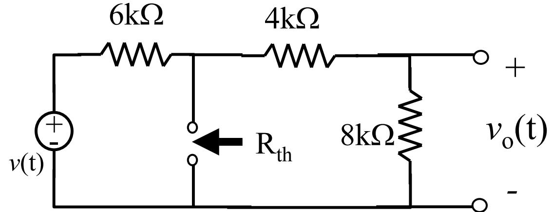
$$R_{th} = 6\text{k}\Omega \parallel (4\text{k}\Omega + 8\text{k}\Omega) = 4\text{k}\Omega$$
