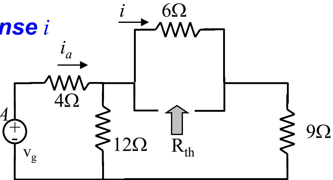
$$R_{th} = (4\Omega \parallel 12\Omega + 9\Omega) \parallel 6\Omega = 4\Omega$$
