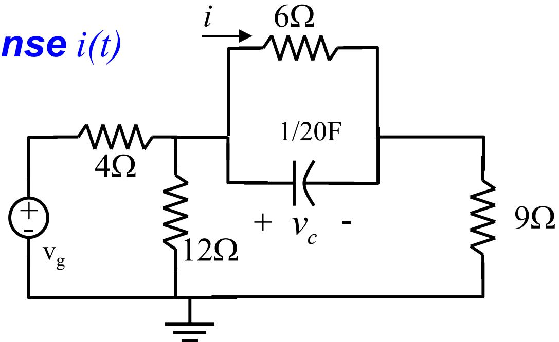
Assume solution of the form:  $i(t) = C_1 + C_2 e^{-\frac{t}{T_C}}$
