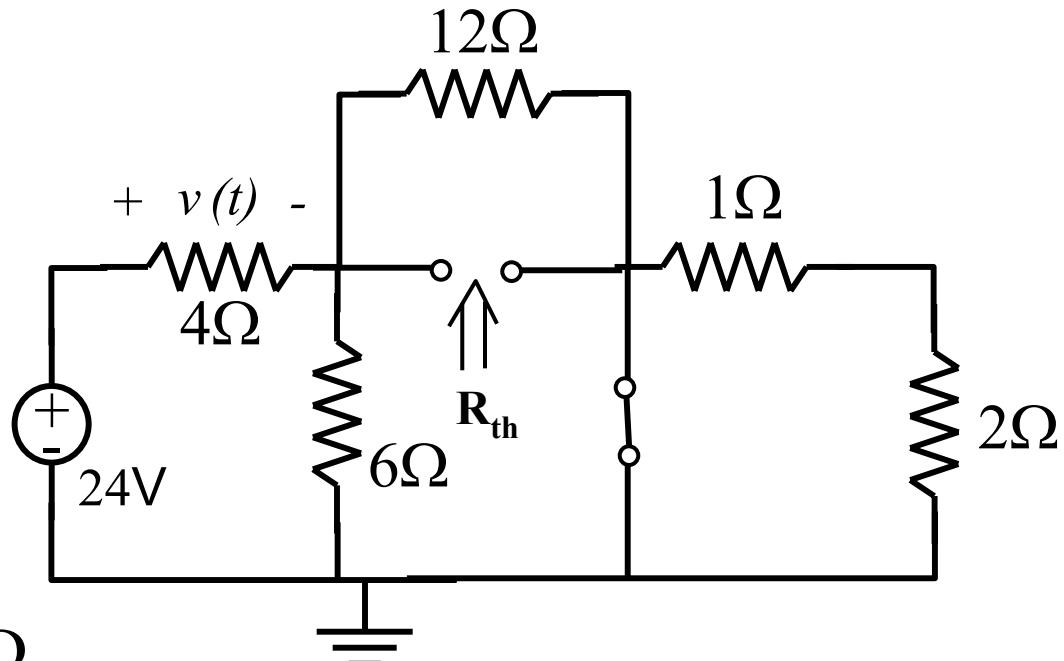
$$R_{th} = 4\Omega \parallel 6\Omega \parallel 12\Omega = 2\Omega$$
