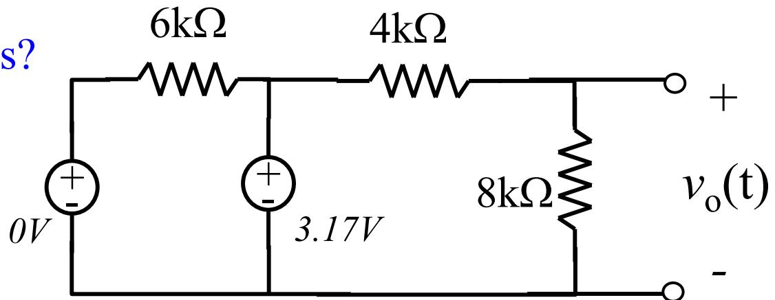
Replace capacitor with voltage source:
