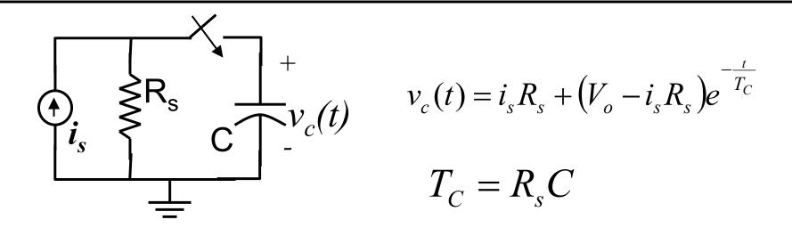
Suppose  $R_s = 1\Omega$   $i_s = 1A$   $V_o = 2V$
