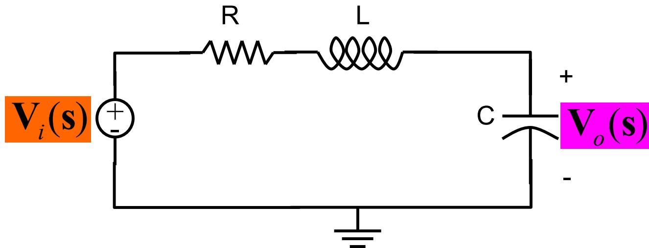
$$V_o(s) = \frac{1/\text{s}C}{R + \text{s}L + 1/\text{s}C} V_i(s) = \frac{1}{LC\text{s}^2 + RC\text{s} + 1} V_i(s)$$
