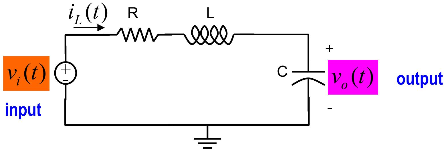
$$\left\{ \begin{array}{l} \text{KCL} \rightarrow C \frac{dv_o}{dt} = i_L \quad \rightarrow \quad C \frac{d^2v_o}{dt^2} = \frac{di_L}{dt} \\ \text{KVL} \rightarrow Ri_L + L \frac{di_L}{dt} + v_o = v_i \end{array} \right.$$
