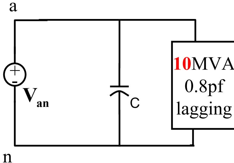
$$S_{\text{old}} = 10 \angle \arccos(0.8) \text{ MVA}$$
