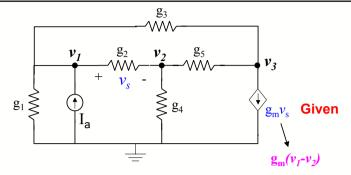
KCL at node 1:  $v_1g_1+(v_1-v_3)g_3+(v_1-v_2)g_2=I_a$
