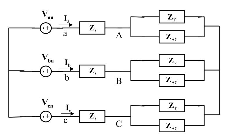
**Per-phase equivalent circuit:**
