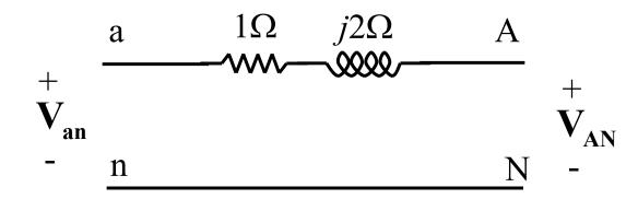
$$\mathbf{V_{an}} = \frac{12}{\sqrt{3}} \angle -30^{\circ} \, kV \, rms \qquad \qquad \mathbf{V_{AN}} = \frac{12}{\sqrt{3}} \angle -25^{\circ} \, kV \, rms$$
