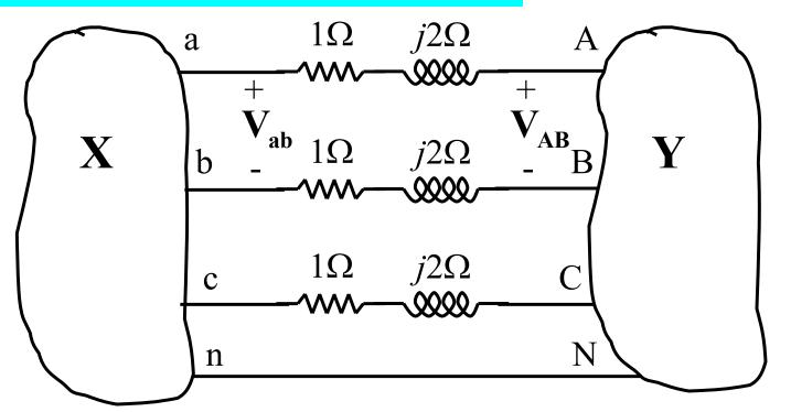
Determine which is the load and which is the source.
