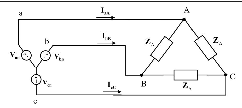
**Phase voltages:**  $V_{AB} = V_{AB} \angle 0^{\circ} = V_p \angle 0^{\circ}$
