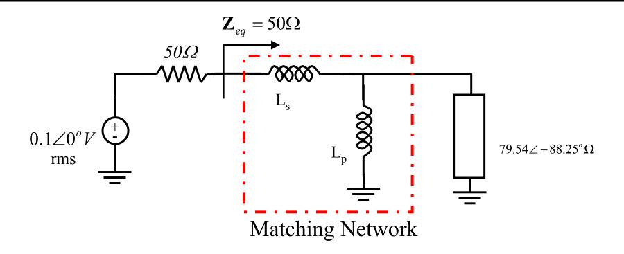
Add a matching network to transform the load impedance, such that the impedance  $\mathbf{Z}_{eq}$  "seen" by the source is  $50\Omega$ .
