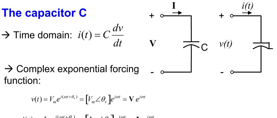
$$i(t) = I_m e^{j(\omega t + \theta_i)} = \left[ I_m \angle \theta_i \right] e^{j\omega t} = \mathbf{I} \ e^{j\omega t}$$
