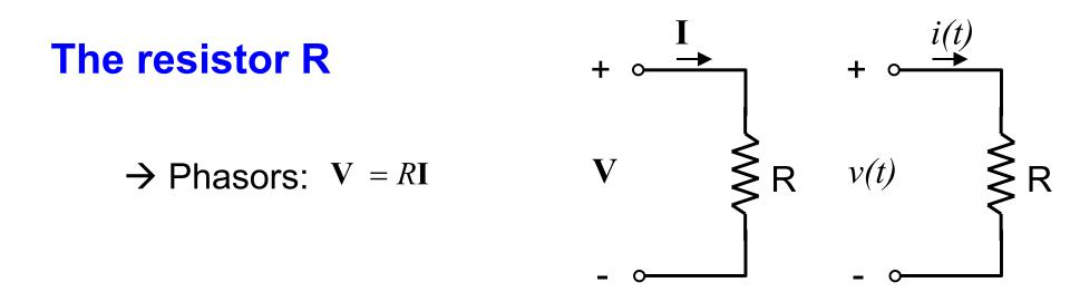
This terminal relation for the phasor voltage and current in a resistor implies that **the voltage and current are in phase**:
