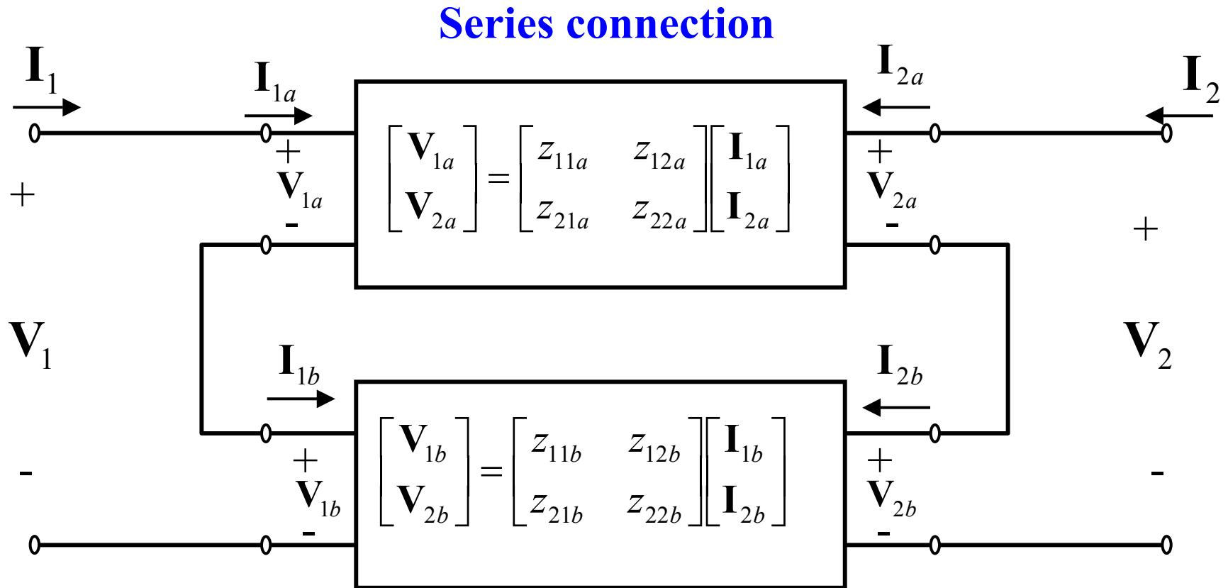
$$V_1 = V_{1a} + V_{1b}$$
