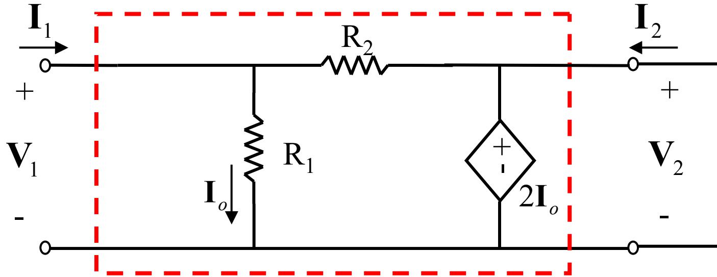
Short circuit test:  $V_2 = 0$
