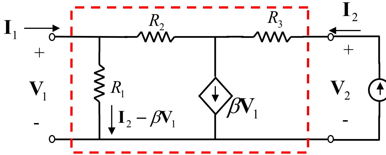
$$V_2(1 + \beta R_1) = (R_1 + R_2 + R_3 + \beta R_1 R_3) I_2$$
