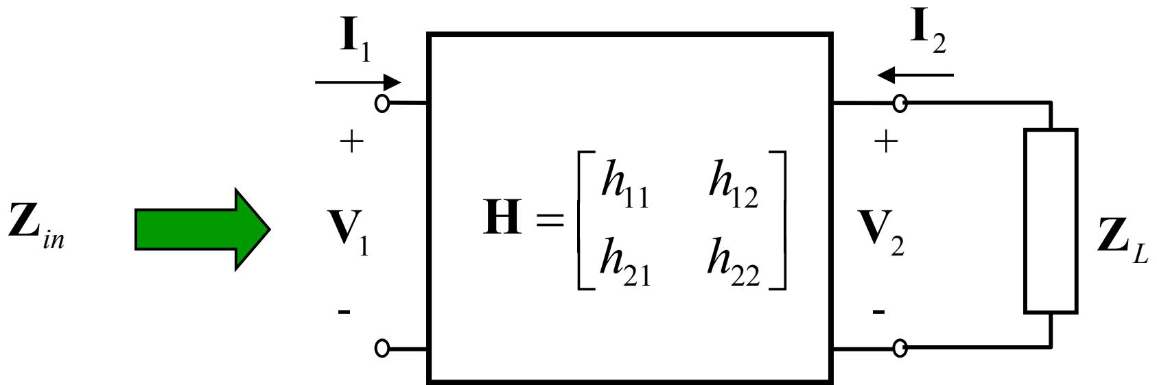
Calculate the input impedance
