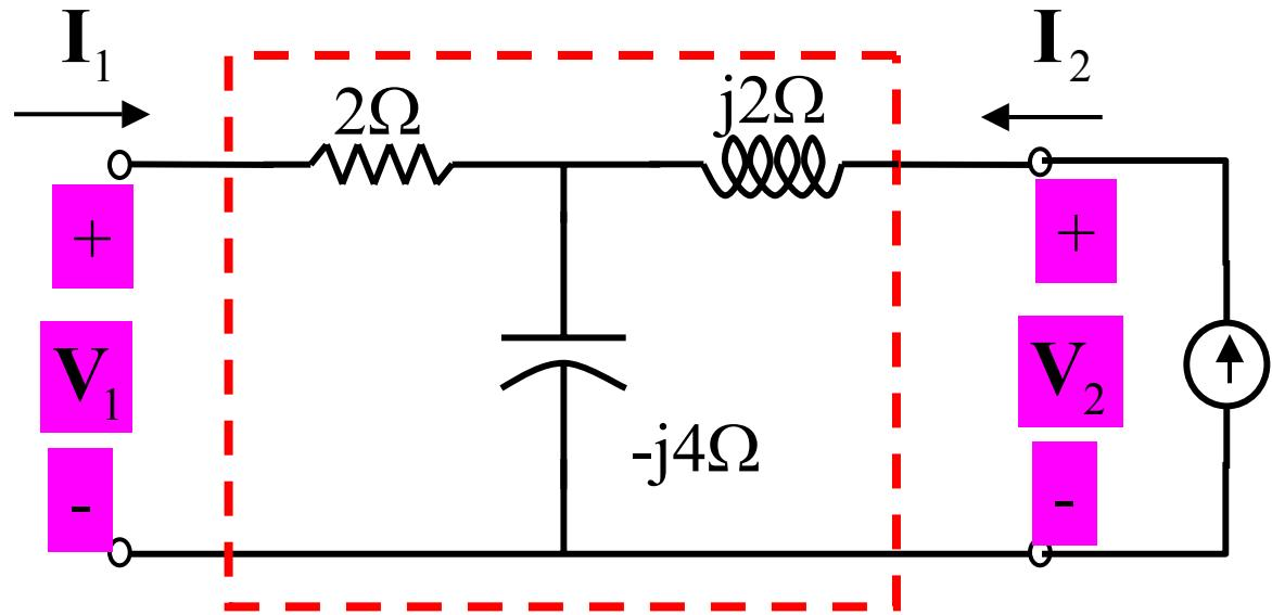
$$V_2 = (2j - 4j)I_2 = -2jI_2 \quad | \quad V_1 = \frac{-4j}{2j - 4j} V_2 = \frac{-4j}{-2j} (-2j)I_2$$
