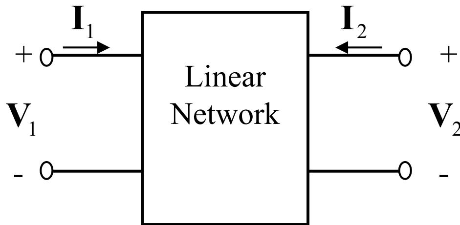
$$\begin{bmatrix} \mathbf{V}_1 \\ \mathbf{V}_2 \end{bmatrix} = \begin{bmatrix} z_{11} & z_{12} \\ z_{21} & z_{22} \end{bmatrix} \begin{bmatrix} \mathbf{I}_1 \\ \mathbf{I}_2 \end{bmatrix}$$
