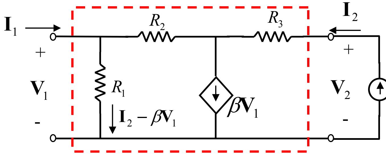
$$V_1 = R_1(I_2 - \beta V_1)$$
