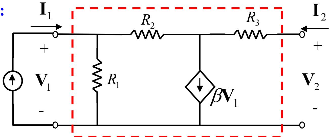
$$I_1 = \frac{V_1}{R_1} + \beta V_1 \quad \rightarrow \quad z_{11} = \left. \frac{V_1}{I_1} \right|_{I_2=0} = \frac{R_1}{1 + \beta R_1} \Omega \quad \textcircled{1}$$
