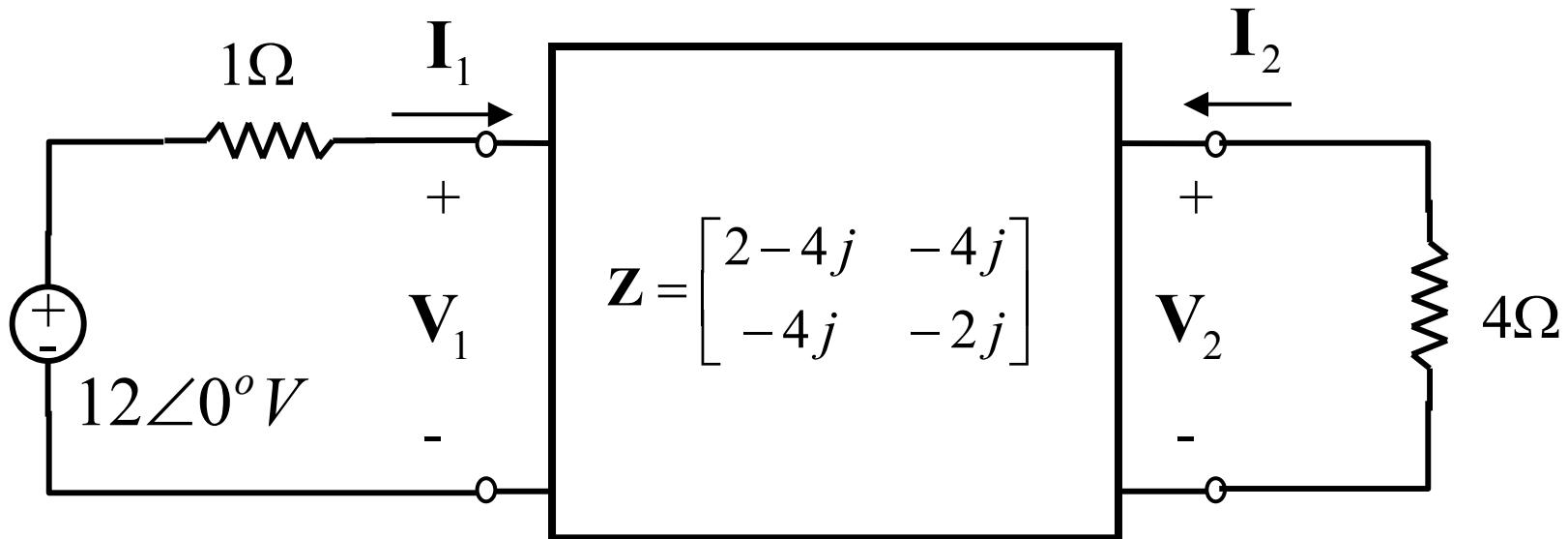
$$\left. \begin{array}{l} V_1 = 12\angle 0^\circ - (1\Omega)I_1 \\ V_2 = -(4\Omega)I_2 \end{array} \right\} \text{Boundary conditions due to terminations.}$$
