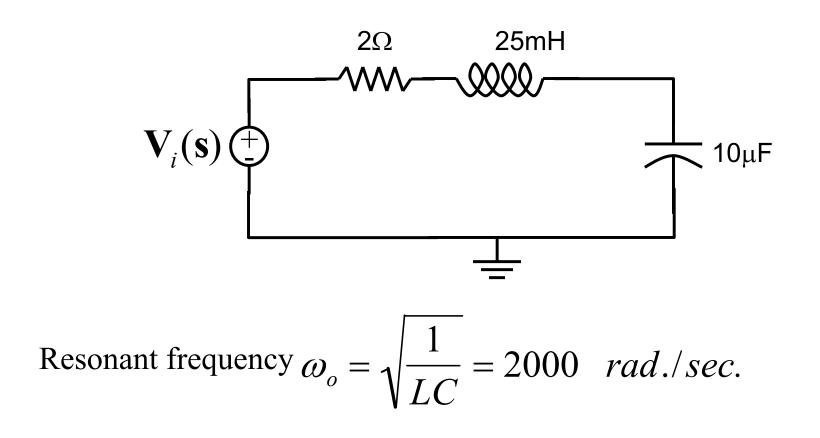
$$Q_o = \frac{\omega_o L}{R} = 25 \qquad BW = \omega_1 - \omega_2 = \frac{\omega_o}{Q_o} = 80 \quad rad./sec.$$
