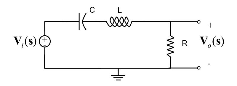
Find R, L and C such that the above circuit operates as a *band-pass* filter with a center frequency of 1000 rad./sec. and bandwidth of 100 rad./sec.
