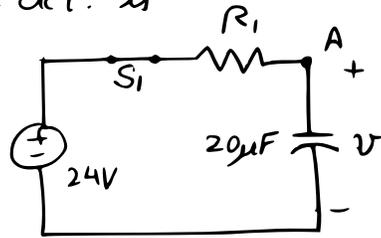
$$-\frac{v}{R_1} + \frac{24}{R_1} = C \frac{dv}{dt}, \text{ or } \frac{dv}{dt} + \frac{1}{RC} v = \frac{24}{R_1 C}$$
