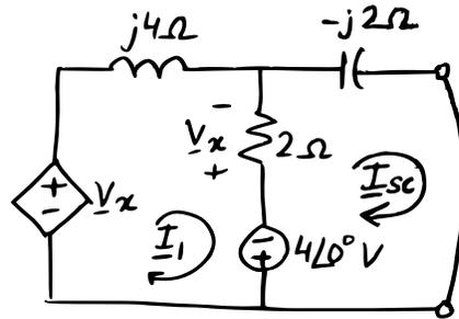
$$j4\underline{I}_1 + 2(\underline{I}_1 - \underline{I}_{sc}) - 4\angle 0^\circ - \underline{V}_x = 0$$
