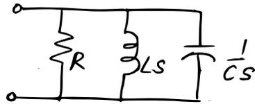
$$Z(j\omega) = \frac{1}{jC\omega + \frac{1}{R} + \frac{1}{jL\omega}} = \frac{\frac{1}{R} - j\left(C\omega - \frac{1}{L\omega}\right)}{\frac{1}{R^2} + \left(C\omega - \frac{1}{L\omega}\right)^2}$$
