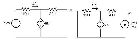
10Io'-8Io'-12=0 2Io'=12 Io'=6 → V'=-48V
