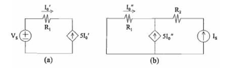
Also: Briefly <u>outline the steps</u> you would take to solve for the power supplied by the voltage source using the superposition circuit solutions for the current "I<sub>0</sub>".
