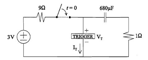
At  $t = 0^-$ , the capacitor is uncharged, the trigger is OFF and the circuit is in steady-state.
