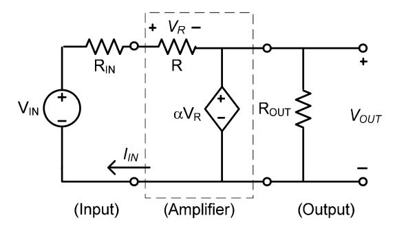
a) Find an expression for the current  $I_{IN}$ , in terms of the parameters  $V_{IN}$ ,  $R_{IN}$ , R and  $\alpha$ .
