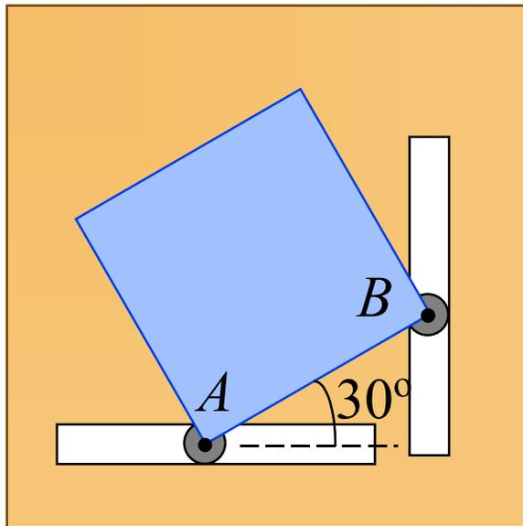
The motion of a square plate of side 150 mm and mass 2.5 kg is guided by pins at corners  $A$  and  $B$  that slide in slots cut in a vertical wall. Immediately after the plate is released from rest in the position shown, determine (a) the angular acceleration of the plate, (b) the reaction at corner  $A$ .
