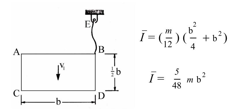
The uniform plate ABCD is falling with a velocity v<sub>1</sub> when wire BE becomes taut. Assuming that the impact is perfectly plastic, determine the angular velocity of the plate and the velocity of its mass center immediately after the impact.
