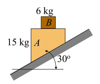
A 6-kg block B rests as shown on the upper surface of a 15-kg wedge A. Neglecting friction, determine immediately after the system is released from rest (a) the acceleration of A, (b) the acceleration of B relative to A.
