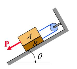
Block *A* has a mass of 30 kg and block *B* has a mass of 15 kg. The coefficients of friction between all plane surfaces of contact are  $\mu_s = 0.15$  and  $\mu_k = 0.10$ . Knowing that  $\theta = 30^\circ$  and that the magnitude of the force **P** applied to block *A* is 250 N, determine (a) the acceleration of block *A*, (b) the tension in the cord.
