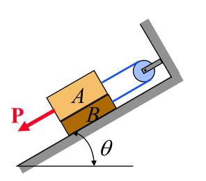
Block *A* has a mass of 30 kg and block *B* has a mass of 15 kg. The coefficients of friction between all plane surfaces of contact are  $\mu_s = 0.15$  and  $\mu_k = 0.10$ . Knowing that  $\theta = 30^\circ$  and that the magnitude of the force **P** applied to block *A* is 250 N, determine (a) the acceleration of block *A*, (b) the tension in the cord.
