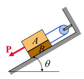
$W_A = m_A g$  $W_A = (30 \text{ kg})(9.81 \text{ m/s}^2)$  $W_A = 294.3 \text{ N}$
