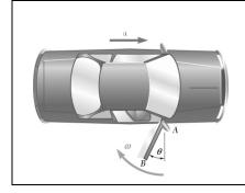
A driver starts his car with the door on the passenger's side wide open  $(\theta = 0)$ . The 36-kg door has a centroidal radius of gyration  $\overline{k} = 250$  mm, and its mass center is located at a distance r = 440 mm from its vertical axis of rotation. Knowing that the driver maintains a constant acceleration of 2 m/s<sup>2</sup>, determine the angular velocity of the door as it slams shut ( $\theta = 90^{\circ}$ ).
