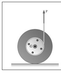
A drum of 100 mm radius is attached to a disk of 200 mm radius. The disk and drum have a total weight of 5 kg and combined radius of gyration of 150 mm. A cord is attached as shown and pulled with a force **P** of magnitude 25 N. Knowing that the disk rolls without sliding, determine (*a*) the angular acceleration of the disk and the acceleration of *G*, (*b*) the minimum value of the coefficient of static friction compatible with this motion.
