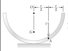
A half section of a uniform thin pipe of mass m is at rest when a force **P** is applied as shown. Assuming that the section rolls without sliding, determine (*a*) its initial angular acceleration, (*b*) the minimum value of the coefficient of static friction consistent with the motion.
