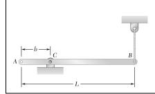
A uniform rod of length L and mass m is supported as shown with b = 0.2 L when the cable attached to end B suddenly breaks. Determine at this instant (a) the acceleration of end B, (b) the reaction at the pin support.
