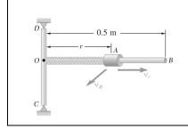
A 2.5 kg collar A is attached to a spring of constant 750 N/m and undeformed length 150 mm. The spring is attached to point O of the frame DCOB. The system is set in motion with r = 250 mm,  $v_{\theta} = 0.5$  m/s, and  $v_r = 0$ . Neglecting the mass of the rod and the effect of friction, determine the radial and transverse components of the velocity of the collar when  $r = 120 \,\mathrm{mm}.$
