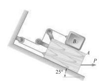
Block A has a mass of 40 kg, and block B has a mass of 8 kg. The coefficients of friction between all surfaces of contact are  $\mu_s = 0.20$  $\mu_k = 0.15$ . Knowing that  $\mathbf{P} = 50 \text{ N} \rightarrow$ , determine (a) the acceleration of block B, (b) the tension in the cord.
