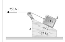
The 15 kg block *B* is supported by the 27 kg block *A* and is attached to a cord to which a 250 N horizontal force is applied as shown. Neglecting friction, determine (*a*) the acceleration of block *A*, (*b*) the acceleration of block *B* relative to *A*.
