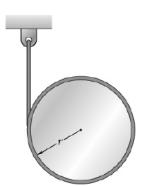
A rope is wrapped around a cylinder of radius r and mass m as shown. Knowing that the cylinder is released from rest, determine the velocity of the center of the cylinder after it has moved downward a distance s.
