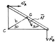
Kinematics. Velocities at A and B are directed as shown. Point C is the instantaneous center of rotation. From geometry,  $b = \frac{L}{2}$ .
